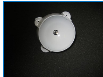
Push the led in from the Back and hot glue in place
