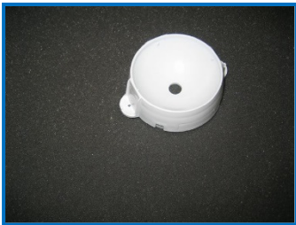
Housing with hole just big Enough for the led
