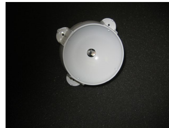
Push the LED in from the back and hot glue in place
