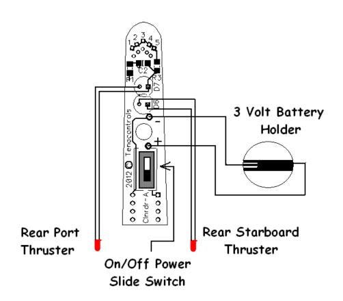
This kit is completely tested for functionality below leaving, so if the rear lights don't work, or the eye is not cycling. Look for a broken wire going to the led or broken wire at the battery holder or at the board connection.
